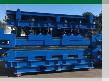
15metric ton Linear Cable Machine designed for stand alone operations laying and recovering large diameter cable in marine environments.
