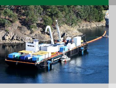
Fully adaptable to meet the needs of the marine construction project as required by the customer. A large platform (67.1 m long x 17.7 m wide) provides ample space for a variety of marine projects.
