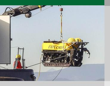
A 25 HP Work Class Electro-Hydraulic Remotely Operated Vehicle (ROV) that can operate to a 1000 metre working depth.
